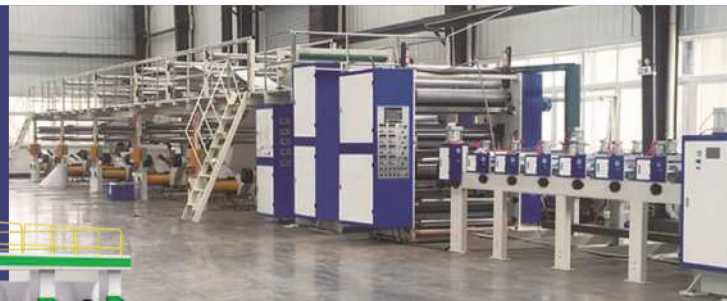
4/5/6 PLY KAPPA BOARD PRODUCTION LINE
